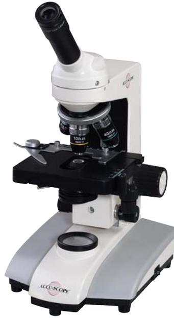
**Stand:** Full size stand with separate coarse and fine adjustment controls set in ergonomic, low positions for comfortable use. Cast alloy aluminum stand with an acid resistant lustrous almond finish and cord hanger.
