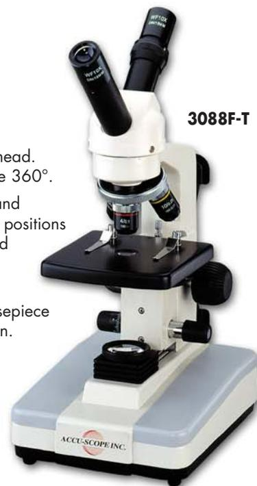
**Head:** Monocular or dual inclined teaching head. Viewing bodies are inclined 45° and rotatable 360°.
